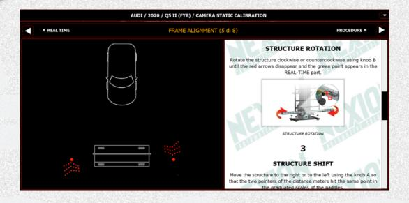
Immediate system positioning is made possible through software real-time data acquisition from different laser pointers.
